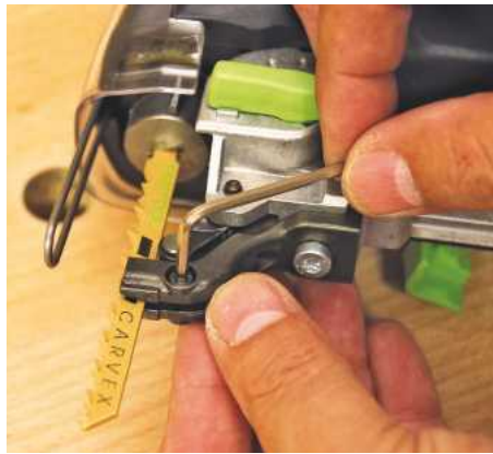
▲ A set of adjustable lower guide blocks gives extra support and minimises drift
